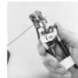
Short-stop latch protects wire strands by limiting the stripping stroke to 5/32" and retains the slug until the wire is ready for terminating
