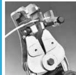
Transparent wire stop provides uniform stripping strength
