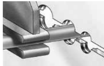
Gripper pads hold the wire securely in a centerline relationship with the blade
